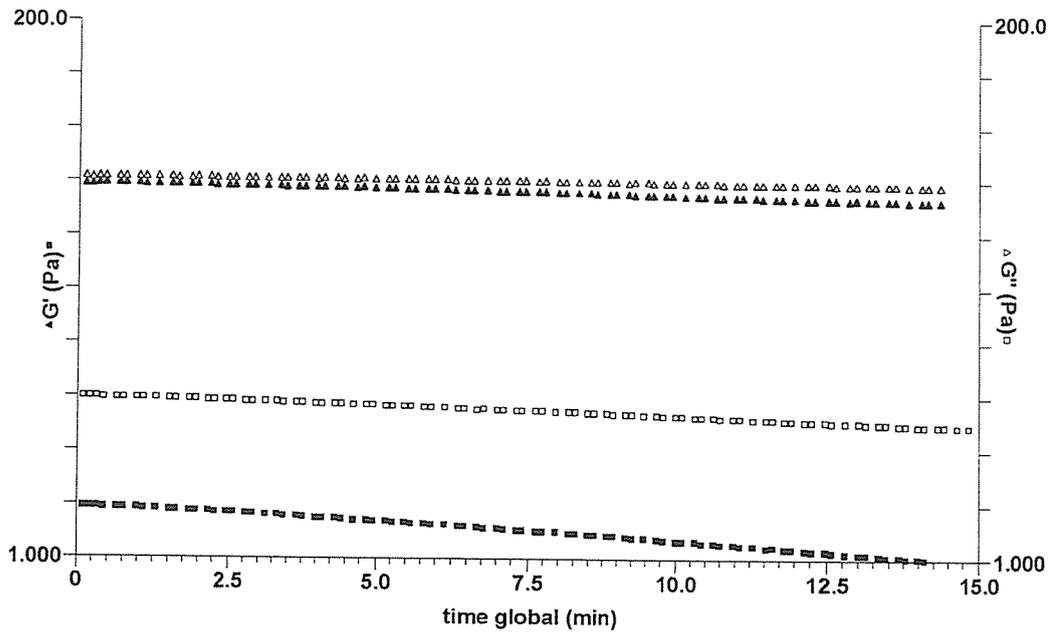
Fig. 1 Elastic ( $G'$ ) and storage ( $G''$ ) moduli at 1 Hz of hyaluronic acid (HA) solutions as a function of oxidative degradation time on linear hyaluronans. *Filled triangle*  $G'$  (Pa) *open triangle*  $G''$  (Pa) on HANOX-M; *filled square*  $G'$  (Pa) *open square*  $G''$  (Pa) on HA 1%
