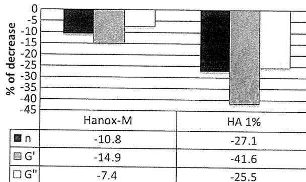
Fig. 2 Decrease (%) of elastic ( $G'$ ) and viscous ( $G''$ ) moduli and complex viscosity ( $|\eta^*|$ ) after 15 min of oxidative stress by hydrogen peroxide. Comparison of two linear non cross-linked viscosupplements: HANOX-M and hyaluronic acid (HA) 1%
