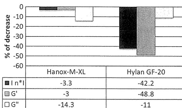
Fig. 4 Decrease (%) of elastic ( $G'$ ) and viscous ( $G''$ ) moduli and complex viscosity ( $|\eta^*|$ ) after 15 min of oxidative stress by hydrogen peroxide. Comparison of two cross-linked viscosupplements: HANOX-M-XL and Hylan G-F 20
